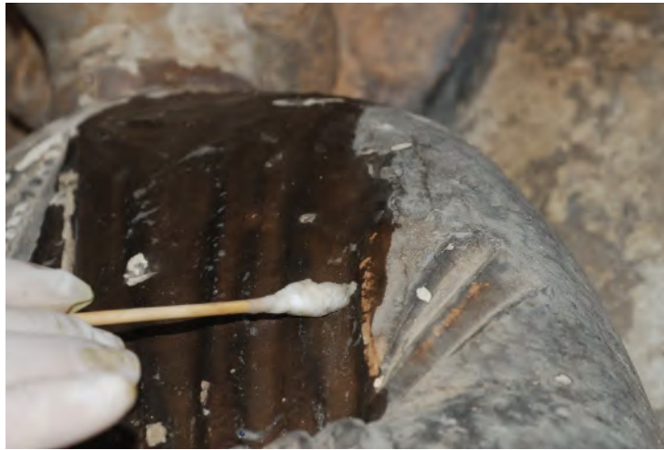
2 Manual cleaning with cotton buds and demineralized water
